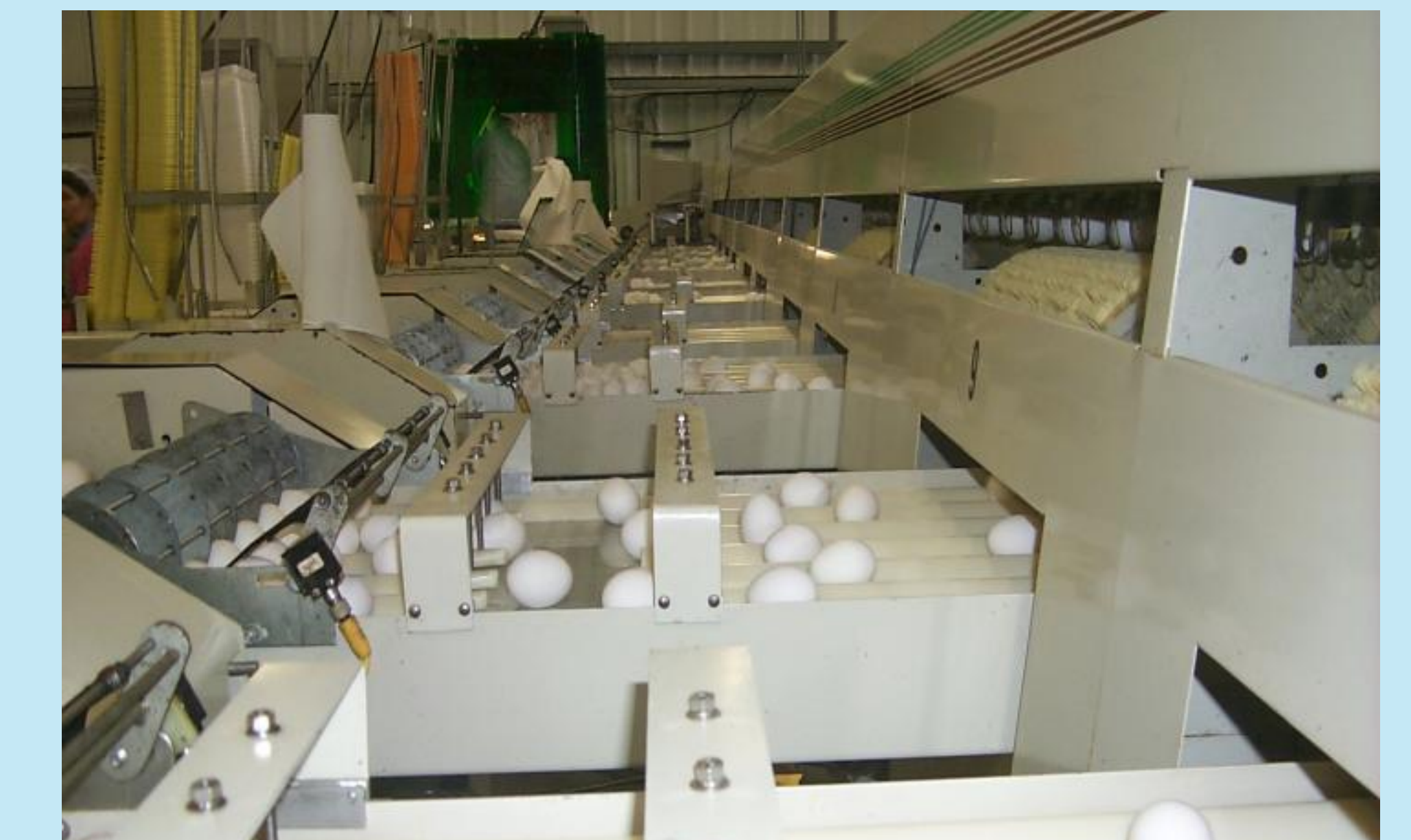
Figure 2. Eggs being directed into foam cartons via packer head brushes and packer lanes in a commercial shell egg facility.
